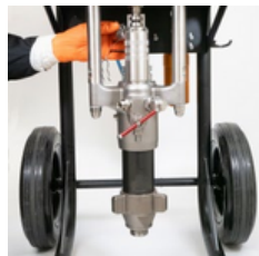
Disconnect the piston collars.
