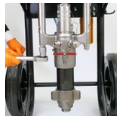
Using a wrench, remove pump from tie rods.
